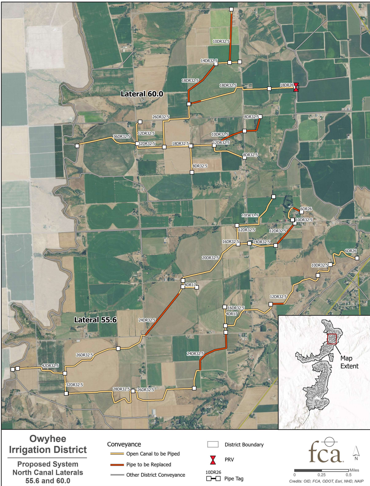
Figure 4-12. Delivery System Improvements – North Canal Laterals 55.6 and 60.0.
